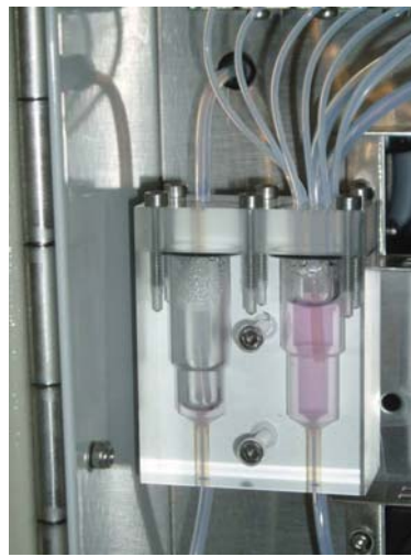
Above: The equipment measures total phosphorus, total nitrogen, nitrate, nitrite, ammonium and phosphate. It can take measurements as frequently as every 15 minutes but is generally set at 1 per hour.
